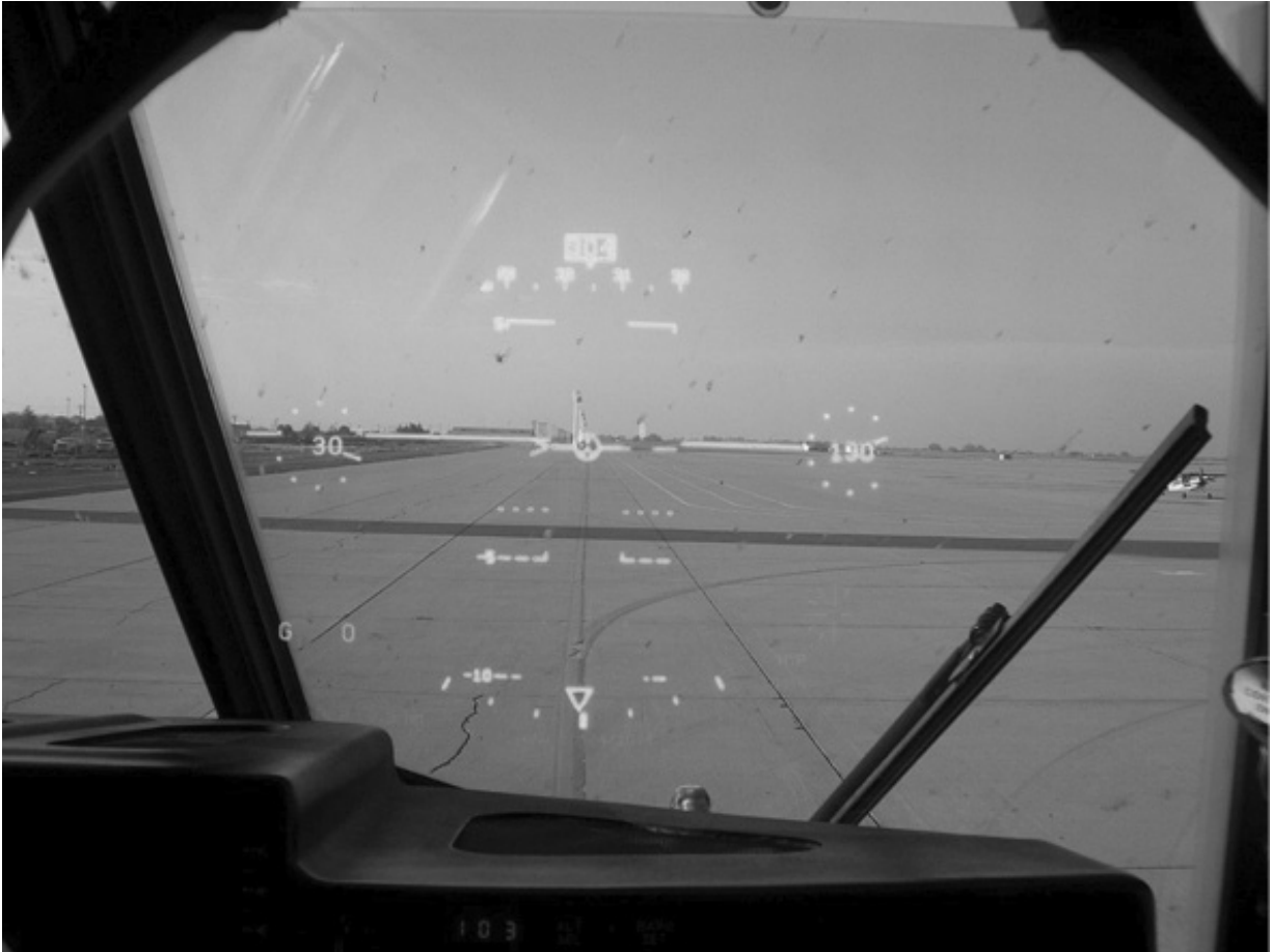
Fig. 4.1. Head-Up Display per copilota di un trasporto aereo Super Hercules. By Telstar Logistics – flickr, CC BY 2.0, https://commons.wikimedia.org/w/index.php?curid=5883242
